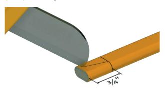
• Remove the exposed grounding braid. Make sure that the insulation jacket is not damaged.
