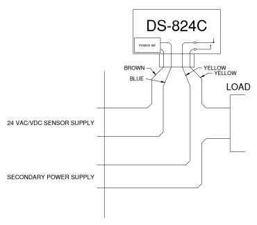
24 VAC/VDC Sensor Supply, Secondary Voltage Out
