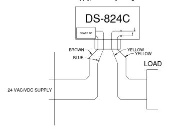
24VAC/VDC Sensor Supply, Dry Contact Thermostat-Style Control
