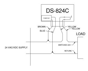
24VAC/VDC Sensor Supply, Supply Voltage Out
